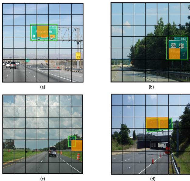
**Fig. 2.** Demonstration of localizing guide panel candidates. The highlighted grids in orange represent where the center of the guide panel falls into, and predict the exact shape of the corresponding bounding box. The green bounding box represents the final regressed shape of the panel prediction. The input resolution of the first layer of the guide panel localization net is  $448 \times 448$ . And the total number of grids is  $7 \times 7 = 49$ . (Color figure online)
