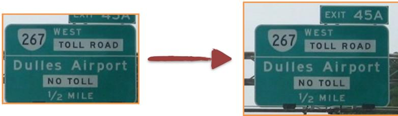
**Fig. 3.** Illustration of the enhancement of initial localized guide panels by extending each edge of the bounding box with 20%.
