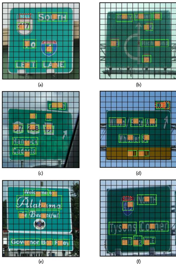
**Fig. 4.** Localization results of the text region candidates within detected traffic guide panels. The highlighted grids in orange predict the exact shape of the bounding box, and represent where the center of the text region candidates fall into. The green bounding boxes represent the finally regressed shape of the text region prediction. The red dashed bounding boxes represent the missed ground truth text region. (Color figure online)
